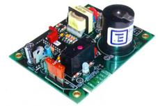
UIB S: 12 volt control board for older furnaces, waterheaters, and refrigerators.
